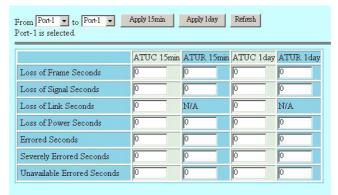
Figure 4-5 DSL Alarm Profile Dialog
